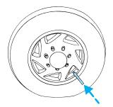
Periodically inspect the tire treads and remove stones, nails, glass or other objects that may be wedged in the tread grooves. Check for holes or cuts that may permit air leakage from the tire and make necessary repairs.
